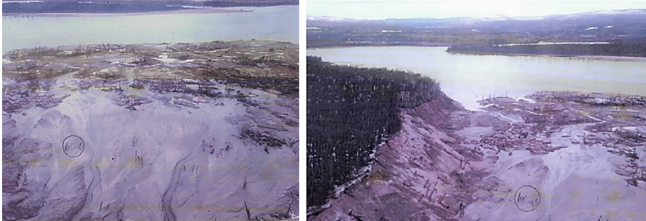
Figure 4.3. The 2014 large landslide south of Muskrat Falls: widening of the Churchill River Valley by large “quick-clay” slides. (Photo: Cabot Martin)
